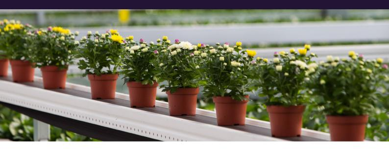
SmartFlo Track conveyor belts convey your pot plants and trays safely and reliably. They have a usable width of 150 or 300 mm, making them an efficient way to transport both plants and trays. The robust conveyor belts can carry static loads, which means the Track can also be used as a walkway.
