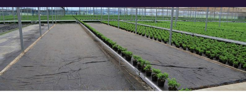
SmartFlo Mobile Tracks are used for carrying pots or trays in and out of a growing compartment. The belts can be handled by two people and can be positioned anywhere. The belts are designed to be easy to extend with further SmartFlo Mobile Tracks. SmartFlo Mobile Tracks are not motorised but are equipped with a connecting axle and a gearbox so that the rotation from the motor can be transmitted to the next belt.
