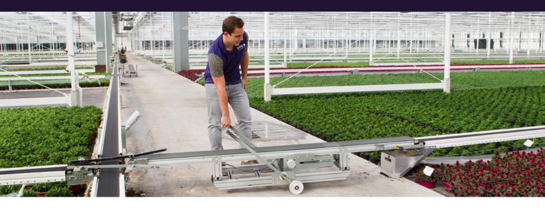
To connect SmartFlo Tracks on either side of the main access aisle, your system can be equipped with a SmartFlo Crossover. This feature does away with the need to cover an unnecessarily long distance to reach the other side of the main aisle: Instead there is just a short, direct route to travel.
