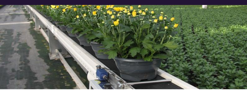
The SmartFlo Stop is a movable, wireless plant stop that is easy to attach at any point along the conveyor belt. When a pot touches the sensor, a signal is sent to the server which shuts down the route. When the pot is removed, the route is automatically restarted and the process resumes.
