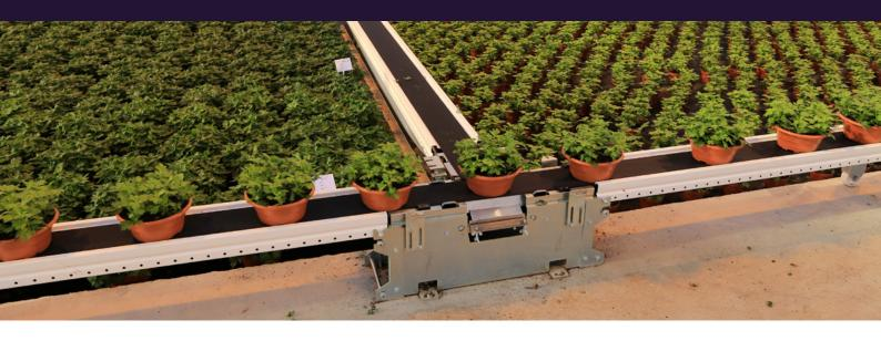
The SmartFlo Extension is an extendible section of belt that can be simply pulled out of a SmartFlo Track in order to connect it to a track on the other side of the main access aisle. It makes no difference how far the SmartFlo Extension is pulled out, it works in every situation.
