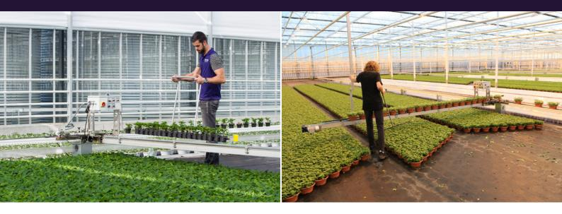
The SmartFlo Flexit provides flexible access to the SmartFlo Track. The SmartFlo Flexit consists of a belt with a mobile connection to the SmartFlo Track, giving easy access to the plants being transported, whether you want to set them down on, or pick them up from, the greenhouse floor. This can be communicated to the route concerned using an integrated SmartFlo Drive.
